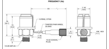
Units on the line drawing are in inches, units in brackets are in millimeters. Refer to 127-3099A5-XX for more information.
